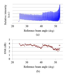
Fig. 11 Results of (a) relative intensity and (b) the SNR of 130 multiplexed holograms.
