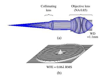
Fig. 13 (a) Optical model for wave aberration analysis and (b) calculated wavefront.
