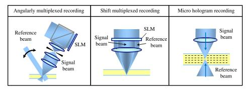
Fig. 1 Representative optical architectures for holographic data storage system.
