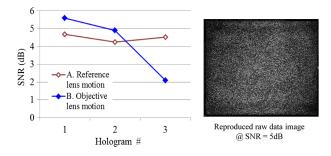
Fig. 8 Measured SNR and reproduced raw data image on camera.
