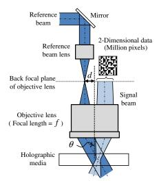
Fig. 2 Overview of monocular architecture.
