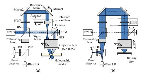
**Fig. 4** Optical architecture for backward compatibility with Blu-ray Disc<sup>™</sup> (BD) system (a) during holographic recording state and (b) during the BD recording/readout state.
