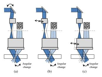
**Fig. 3** Monocular architecture, angular multiplexing by (a) mirror tilt, (b) reference beam lens shift, and (c) objective lens sift.
