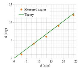
Fig. 6 The result of output angle of reference beam with respect to the optical axis of the objective lens.
