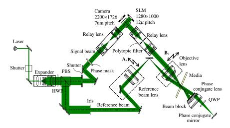
Fig. 5 Monocular experimental setup using green laser system and low numerical aperture (NA) objective lens.
