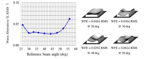
Fig. 12 Wave aberration of various incident angles of reference beam at 26, 36, 48, and 56 deg calculated by ray tracing.
