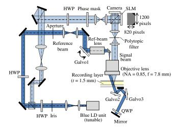
Fig. 10 Monocular test-bed composed of a blue laser system and objective lens of NA 0.85.
