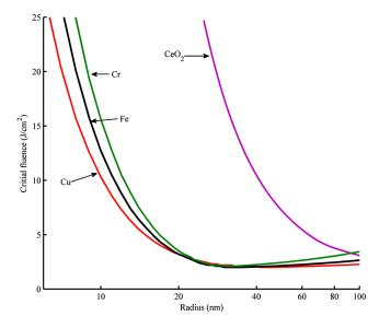
Fig. 2 Critical fluence calculated as a function of particle radius for various particles.
