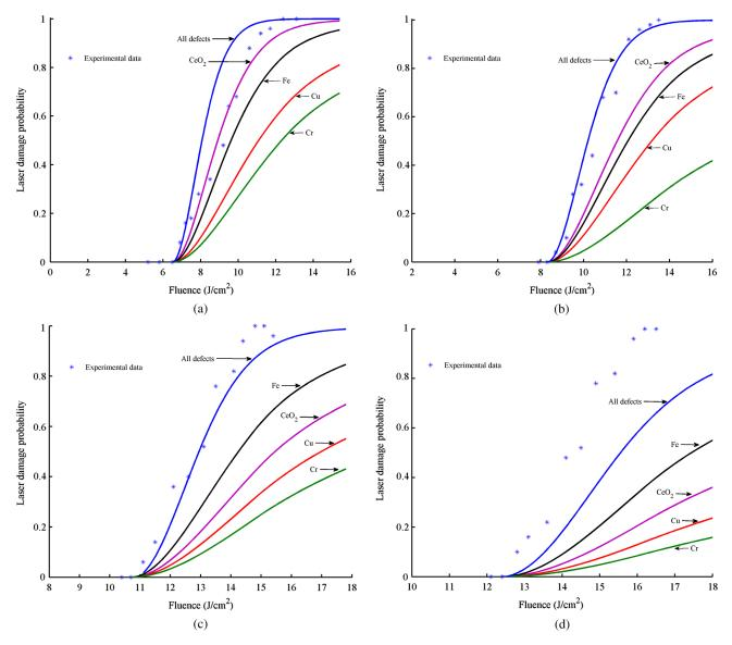
**Fig. 6** The data points of damage probability measured on the surface of fused silica and theoretical curves initiated by impurities for different samples. (a) S1. (b) S2. (c) S3. (d) S4.
