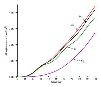
Fig. 1 The absorption cross-section calculated at 355 nm as a function of particle radius for various particles.
