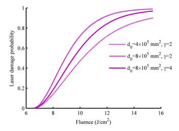
**Fig. 3** Laser damage probability initiated by CeO<sub>2</sub> particles with different distribution parameters  $d_0$  and  $\gamma$ .
