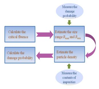
Fig. 5 The scheme for calculating damage probability.
