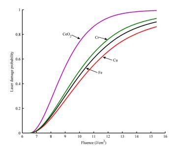
**Fig. 4** Laser damage probability initiated by various particles with same distribution parameters ( $d_0 = 1 \times 10^6 \text{ mm}^2$  and  $\gamma = 3$ ).
