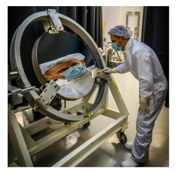
Fig. 8 Picture of  $\phi$ 800 mm 90-deg off-axis parabola with a high laser resistance coating for multi-PW laser systems.
