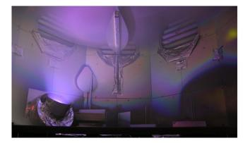
Fig. 2 The RF ion source.
