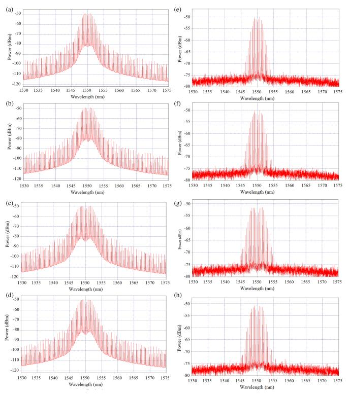
Fig. 4 Received spectrum (a–d) before SMF and (e–h) after SMF, when  $\alpha = 0.14, 0.12, 0.11, and 0.1$ .
