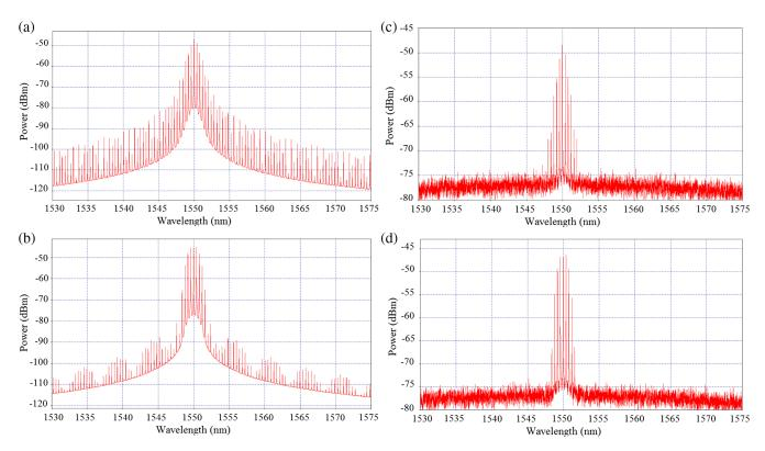
Fig. 3 Received spectrum (a, b) before SMF and (c, d) after SMF, when the DC bias 0.5 and 2.9 v.
