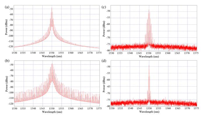
Fig. 2 Received spectrum (a, b) before SMF and (c, d) after SMF, when the amplitude of the sinusoidal is 0.5 and 2.9 v.
