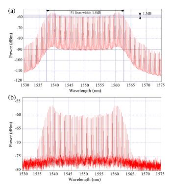
Fig. 5 Received spectrum (a) before SMF and (b) after SMF, when  $\gamma = 0.1$ .
