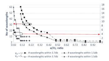
Fig. 6 Relation between number of generated wavelengths and  $\gamma = \alpha/V_{\pi}$  ratio.
