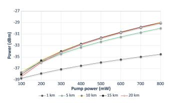
**Fig. 7** Relation between the generated wavelengths power and Raman pump power at different fiber length.
