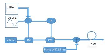
Fig. 1 Configuration of multiwavelength lasing (CW-LD, continuous wave-laser source; IM, intensity modulator; PM, phase modulator; and PS, phase shift).
