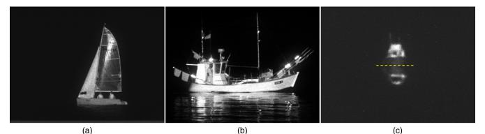
Fig. 35 (a) GV images (M506) of maritime targets showing the capability for target segmentation, (b) indirect specular reflections, and (c) mirage effect at longer distances.
