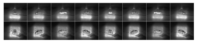
**Fig. 19** Measurement of the laser reflectance signature of a civilian target for different target aspect and sensor elevation angles. Top row: sensor elevation of 0 deg. Bottom row: sensor elevation of 20 deg. Columns: target aspect angles of 0, 45, 90, 135, 180, 225, 270, and 315 deg (from left to right).
