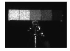
**Fig. 18** GV image (M506) of five diffuse reflectance targets consisting of Spectralon and mounted on a tripod for field application. The edge length of each square board is 20 cm.
