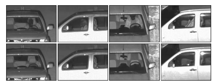
**Fig. 42** Cropped, active SWIR images at  $\lambda = 1.55 \,\mu$ m of a vehicle with person (top row) and without person (bottom row) at the wheel. The sensor elevation angle is 0 deg (first and second column) and 20 deg (third and fourth column). The target aspect angle is 0 deg (first and third column) and 90 deg (second and fourth column).
