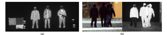
**Fig. 33** (a) GV image (M506) of four reference targets and three persons wearing different clothes for the purpose of measuring the laser reflectance of the clothes at  $\lambda = 1.57 \ \mu$ m. (b) Visual and GV image (M506) of persons with high reflecting clothes except one very low reflecting pair of trousers.
