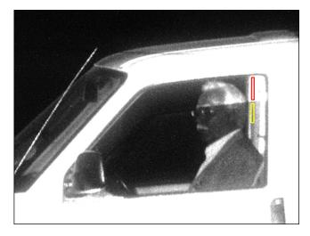
**Fig. 41** GV image (M506) of a person sitting in a vehicle with partially opened window. Two rectangles indicate ROIs for estimation of laser transmission.
