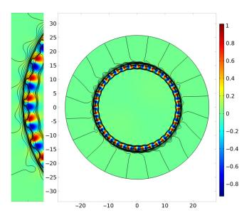
**Fig. 4** Distribution of the transverse Poynting vector component projection on the radius vector direction in the silica glass segmented capillary cross section (N=36). The streamlines for the transverse component of the Poynting vector (black lines). All dimensions are in  $\mu$ m.
