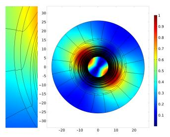
**Fig. 3** Distribution of the transverse Poynting vector component projection on the radius vector direction in the silica glass capillary cross section. The streamlines for the transverse component of the Poynting vector (black lines). All dimensions are in  $\mu$ m.
