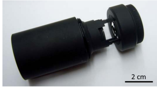
Fig. 9 Photograph of the 3:1 scale prototype. Four pillars are used to connect the front and back optics groups instead of using transparent housing. The entire device is 7 cm long and 3 cm in diameter.
