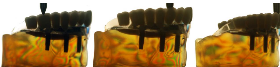
Fig. 2 Stress distribution in the model with splinted implants with a bar connected to distally placed O-rings (cantilever) (BOD).
