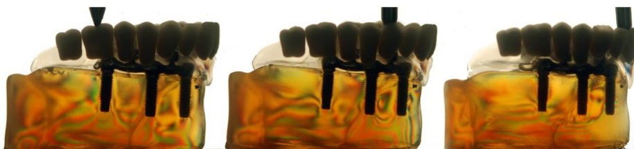
Fig. 1 Stress distribution in the model with splinted implants with a bar connected to centrally placed O-rings (BOC).
