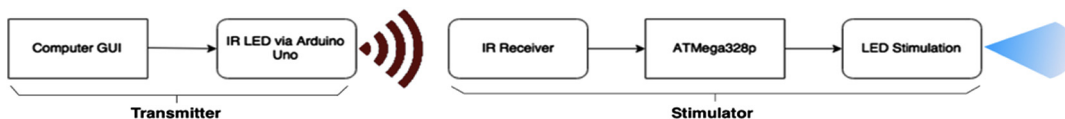
Fig. 4 The flowchart demonstrating CerebraLux activation. The computer GUI is connected to an Arduino Uno-controlled IR LED. After pressing “activate LED” on the GUI, the transmitter sends IR pulses to the head-mounted module, where it is received by the photodiode and sent to the ATmega328p microcontroller for processing. The microcontroller then outputs the desired on-time, off-time, and light intensity to the LEDs for stimulating the region of interest in the mouse brain.
