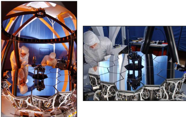
Fig. 17 The test bed telescope is a scaled replica of The James Webb Space Telescope, having full sensing and control functionality.
