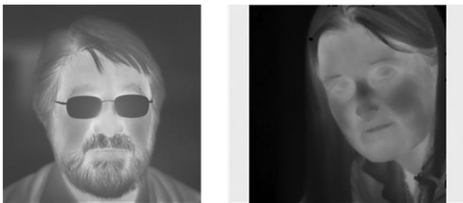
Fig. 8 The infrared image on the left is taken by L3 from a 1024 \times 1024 FPA. The image on the right is taken by MIT Lincoln Lab from a 256 \times 256 FPA.
