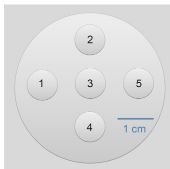
Fig. 2 Sample layout of a typical 2-in. silica sample used for \rho(\phi) damage testing.
