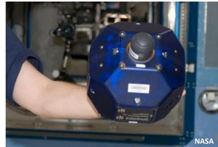
Figure 8: SPHERES Module
