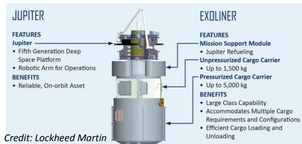
**Figure 7:** Jupiter ExoLiner Servicing Concept
