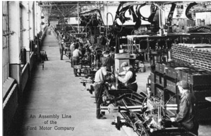
Figure 1: Ford Motor Company Assembly line in 1913. The accelerating speed with which Ford could produce cars helped him continue to lower the price of the Model T. 2
