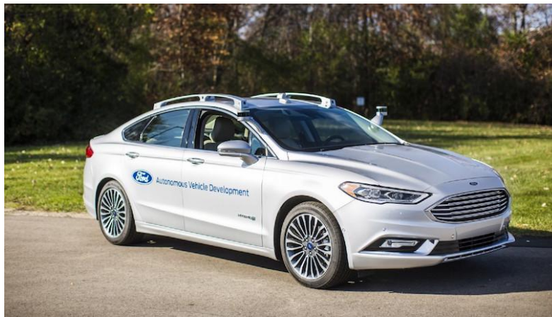
Figure 5: Ford's autonomous vehicle development with integrated LiDAR. 13
