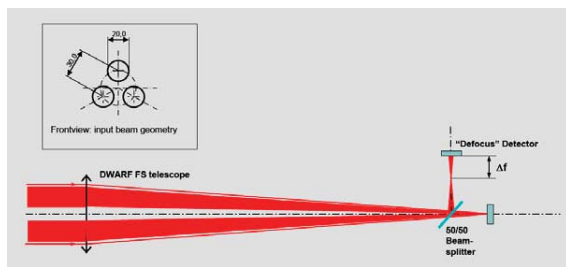
Fig. 2. Schematic diagram of the FS BB. A telescope focuses three incoming beams on the Fringe Sensor detector unit, where one focused and one defocused interference fringe are detected.
