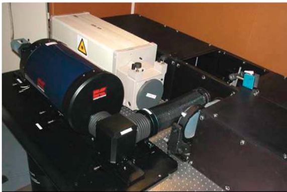
Fig. 7. The DWARF BB is installed on the BRISE test bench ready for testing; the optical path is closed with baffles to suppress any stray light.
