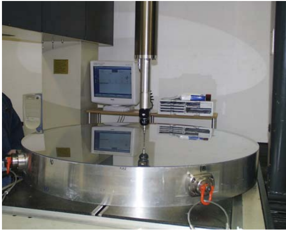
Fig. 6. Surface error measurement with CMM
