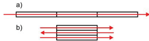
Figure 3. PO risk reduction: a) long medium, b) wide medium with triply folded beam
