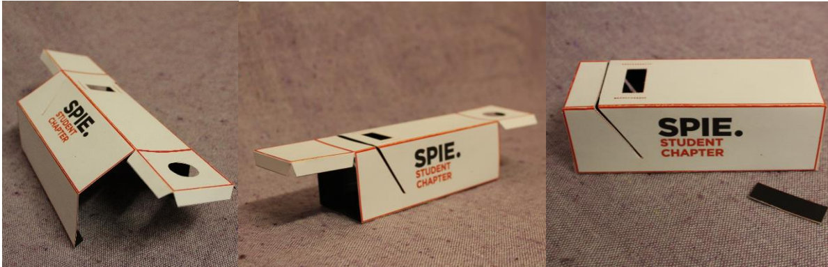
Figure 12. Bend and stick the template. Do not forget to fit the shutter in the slits.
