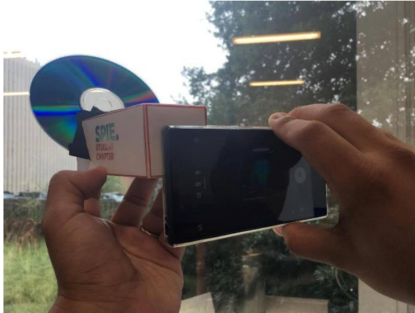
Figure 14. Use your phone to take pictures of the spectra that you obtain from different sources.
