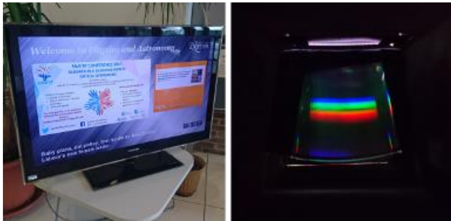
Figure 20. An LCD screen contains pixels that can produce only three colors: red, blue and green. All the colors that you can see in the screen are a mixture of these three. The spectrum a LCD screen just contains those three colors.
