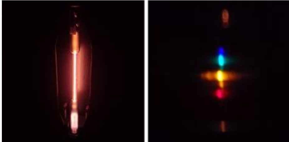
Figure 21. The spectrum of a helium lamp. Excited atoms produce spectra because their atoms have electrons in different energy levels. Electrons moving from a high energy level to a lower energy level produce light with different wavelengths, or colours.
