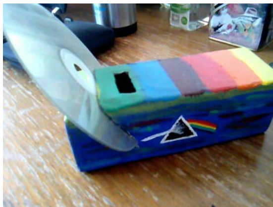
Figure 6. An unfinished homemade spectrometer built by students from a Chilean high school. They modified the external design to make it unique.
