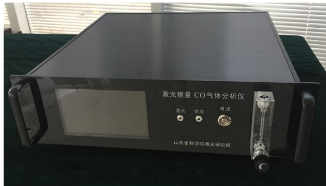
Figure 3. The engineering prototype of CO monitoring system.
