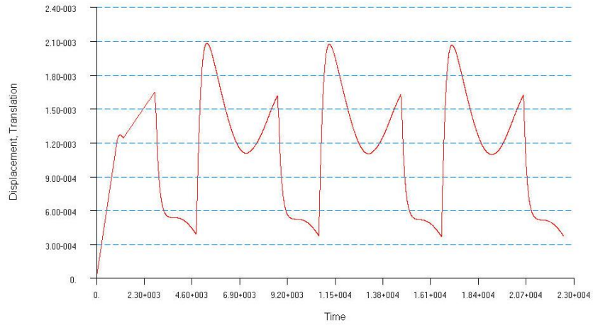
Fig.8. Displacement versus time curve of the center position of flexible structure
