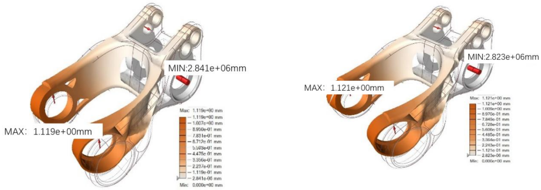
(a) shift 1.119mm of carbon fiber modified polyester material (b) displacement 1.121mm of glass fiber composites
