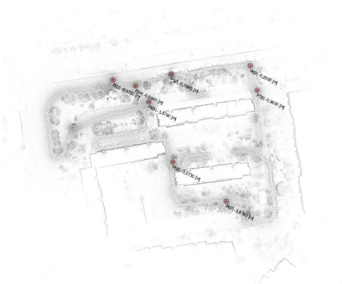
Figure 8. Georeferencing in GeoSLAM Draw, using the coordinates of the ground points from the photogrammetric models
