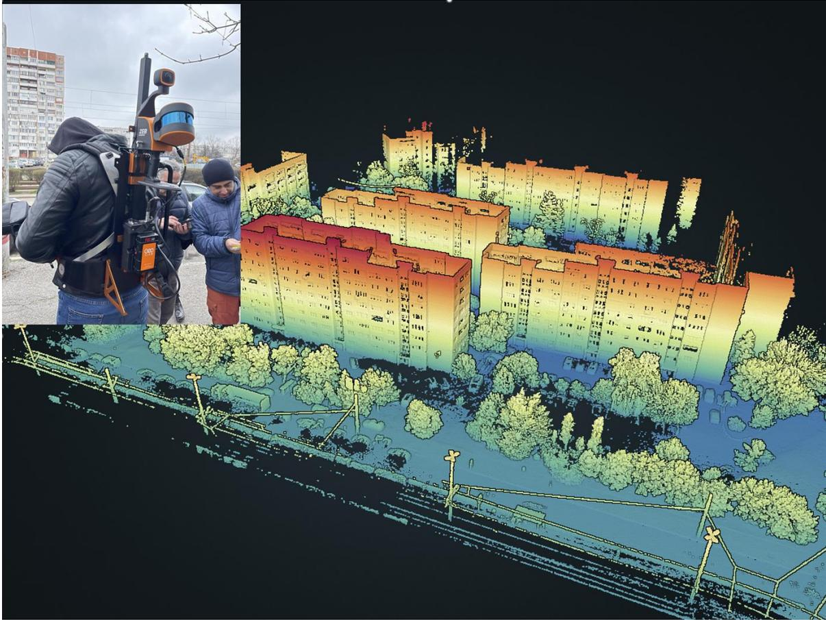
Figure 7. Results from ground laser scanning with a backpack-mounted ZEB Horizon geoSLAM
