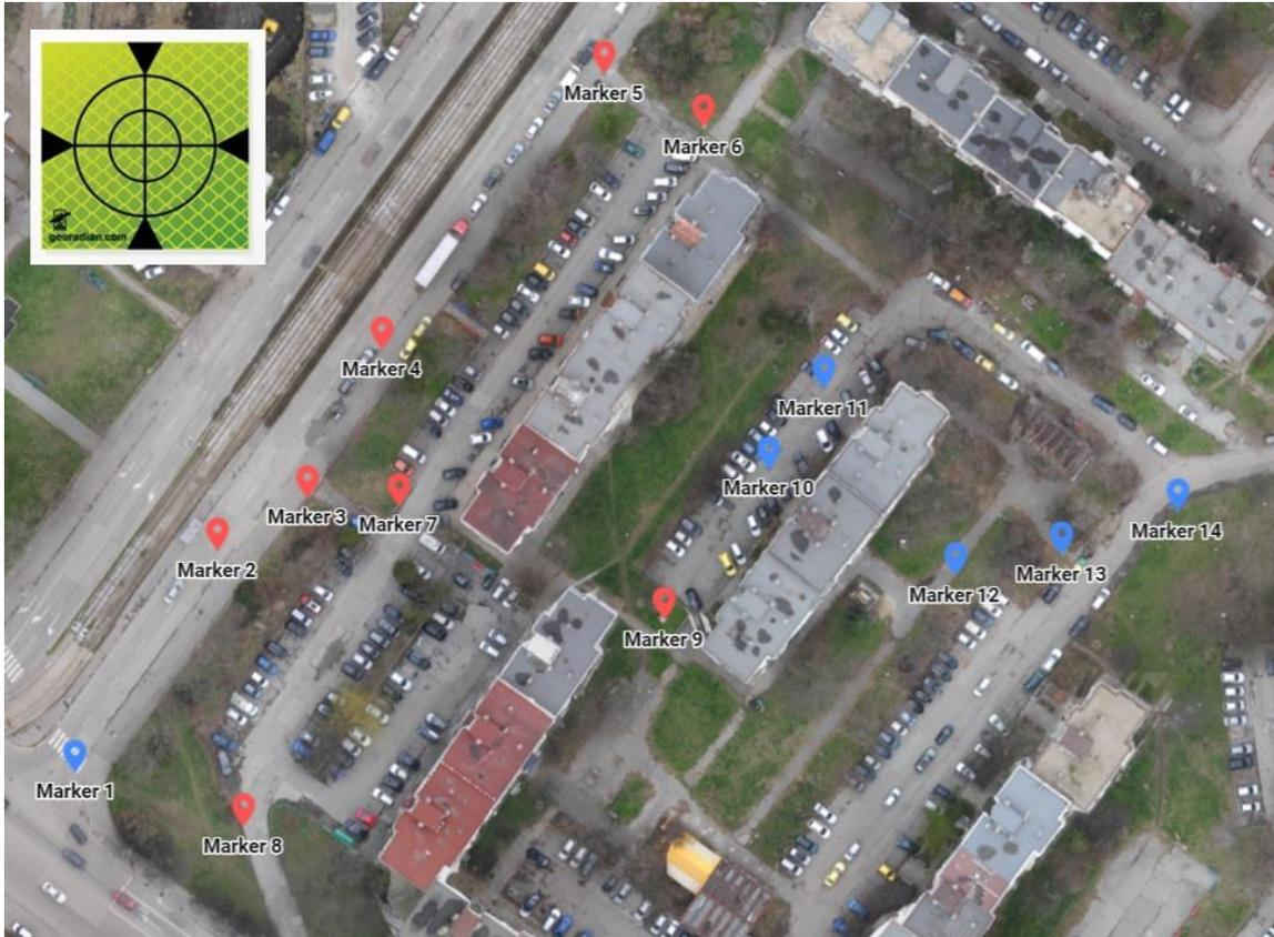
Figure 4. Control points marked with reflective signs on the area. The red points on the map are controlled via GNSS measurements
