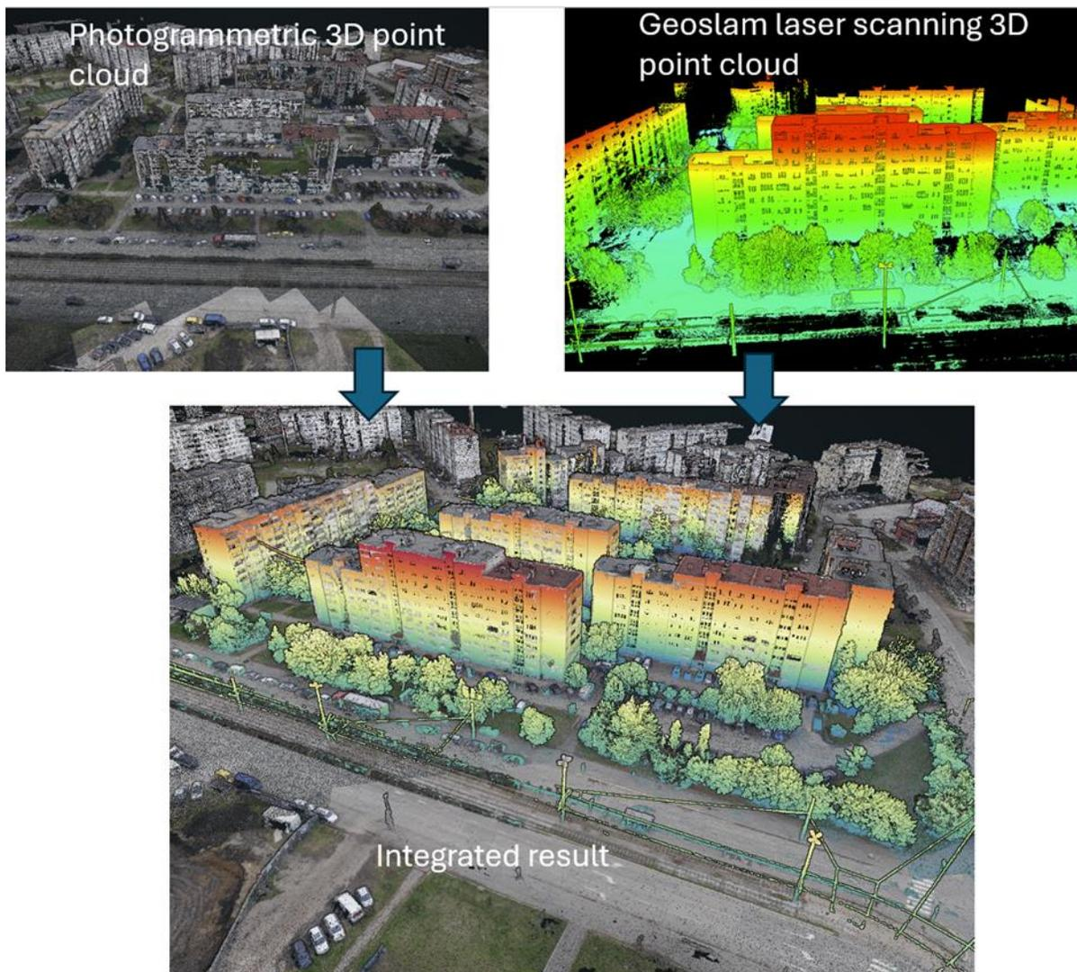
Figure 9. Integrated digital model of the urban area under study
