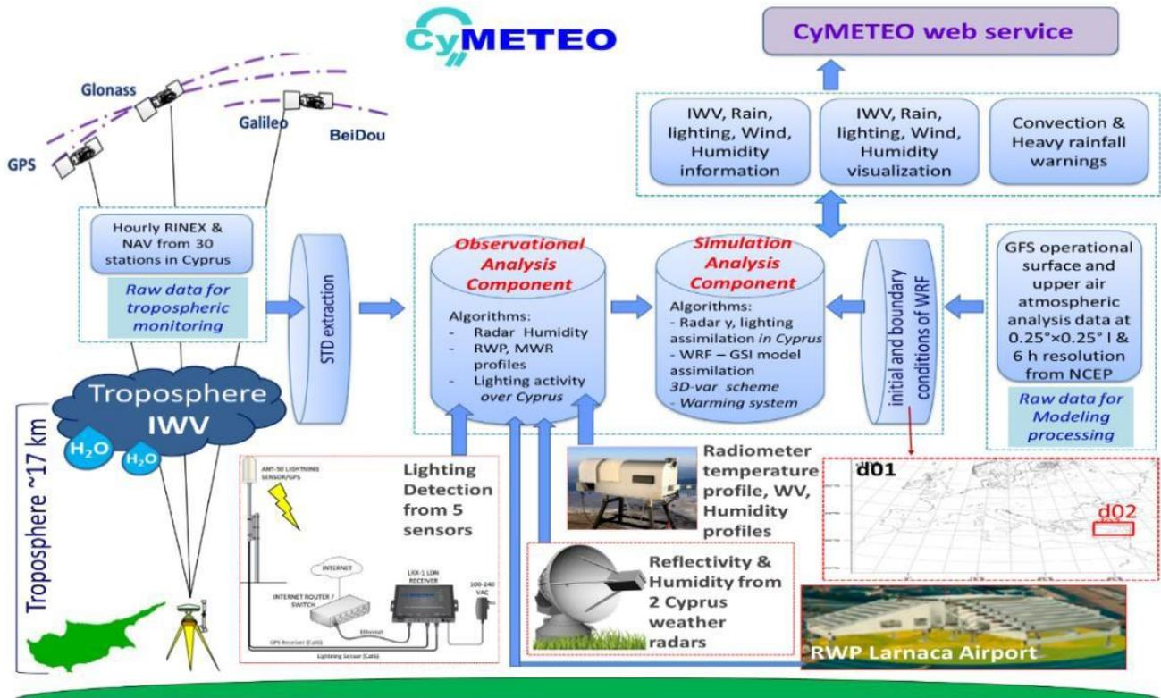
Figure 2. CyMETEO system architecture in the frames of CYGMEN project.
