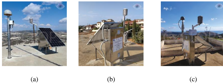
Figure 4: CyCLOPS GNSS Mobile Stations at Pissouri, where (a) CUT300CYP, (b) CUT400CYP and (c) CAVO00CYP
