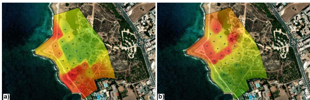
Figure 6. Results from the laboratory showing where lower and higher concentrations of Conductivity ( \mu\text{S}/\text{cm} ) and Acidity (pH) exist. The left-side image (a) shows Conductivity ( \mu\text{S}/\text{cm} ) levels. Red color indicates higher concentrations of conductivity, and green indicates less concentration of conductivity. The right-side image (b) shows Acidity (pH) levels. Red color indicates higher concentrations of acidity, and green indicates less concentration of acidity.
