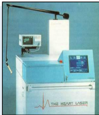
Figure 5: The Heart Laser – this laser system was sold by PLC, MA and contained a fast axial flow laser from TRUMPF. TRUMPF was asked to develop a diffusion cooled CO 2 laser to replace the fast axial flow laser in 1996.
