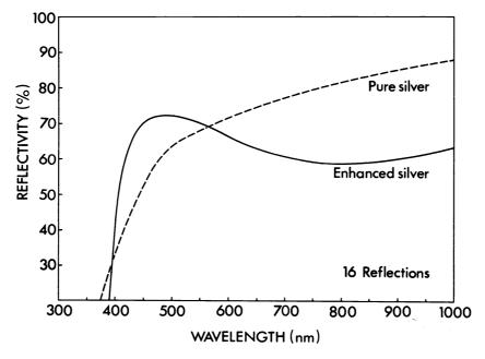
Figure 2 Reflectivity of 16 Surfaces Using Enhanced Silver Coatings
