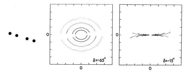
Figure 3 (u,v) Plane Coverage for the Linear Array Shown (tilted 15° to the E-W Direction) to the Left. Maximum Zenith Distance is 60°.
