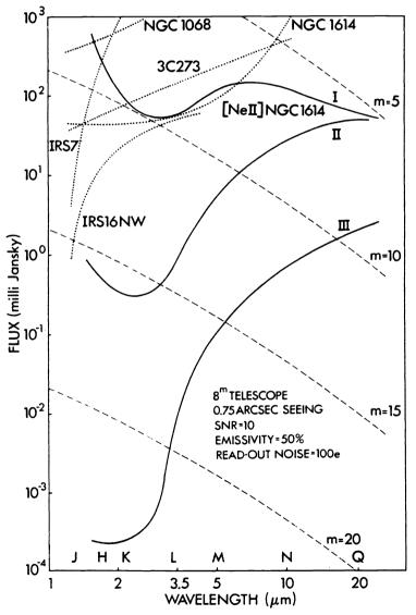
Figure 1 Sensitivity Estimates for the 8 meter VLTI Array (see text)
