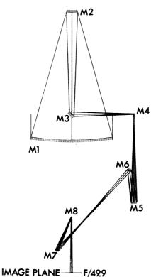
Figure 6 Coudé Feed Optics for the 8 Meter Telescopes (Shown to Scale) 3.3 <u>Coudé Relay Optics</u>
