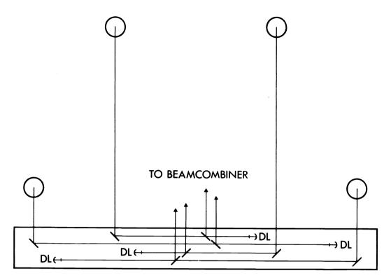
Figure 8 Transfer Optics Between the Coudé Optics of Each 8 meter Telescope and the Beamcombiner (BC) Consist of Three 90° Reflections (last one into BC not shown) and a Delay Line (DL)
