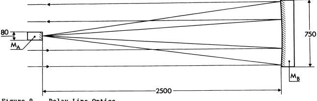
Figure 9 Delay Line Optics
