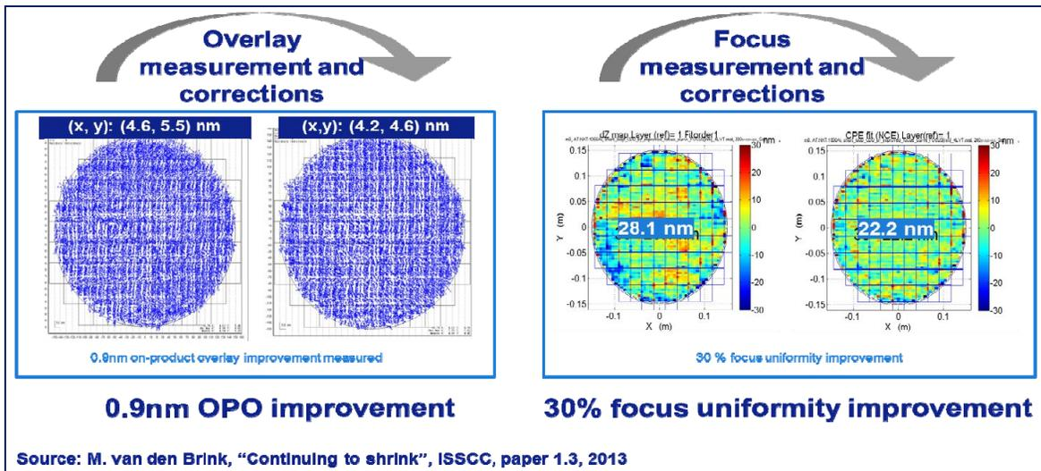
Figure 10: Integrated metrology can improve on-product overlay and focus.
