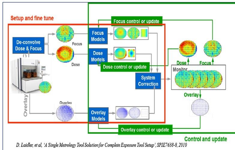
Figure 4: A single metrology tool solution for focus, dose and overlay scanner setup [13].
