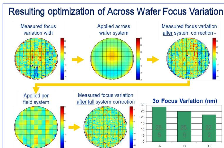
Figure 5: Resulting optimization of across wafer focus variation [13].
