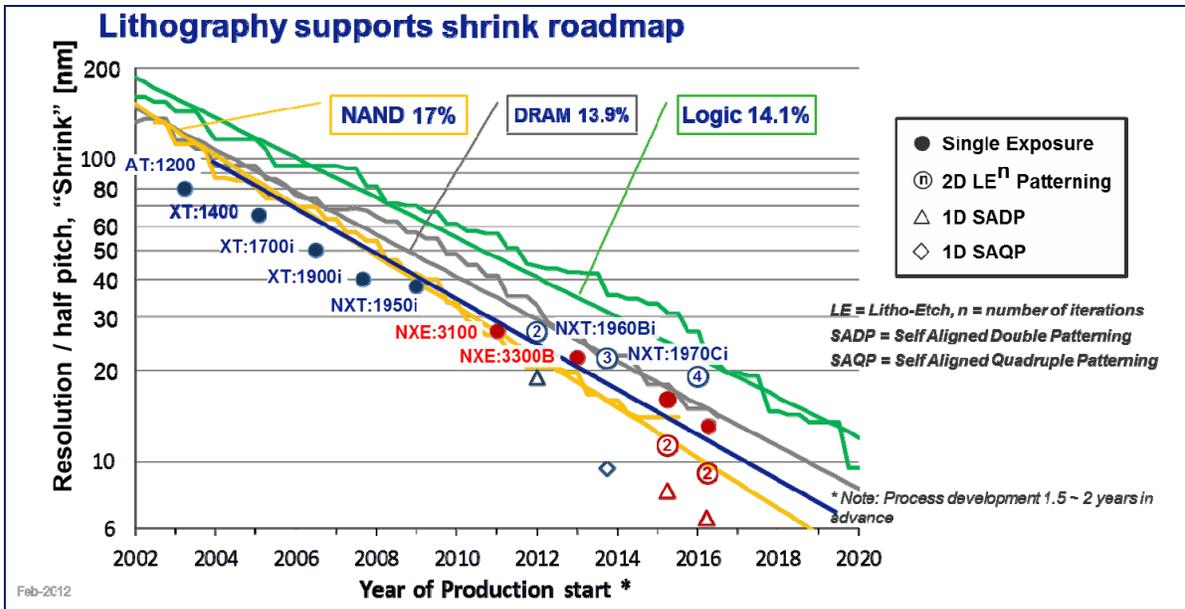
Figure 1: Industry roadmap towards <10nm resolution. Lithography supports the shrink roadmap.
