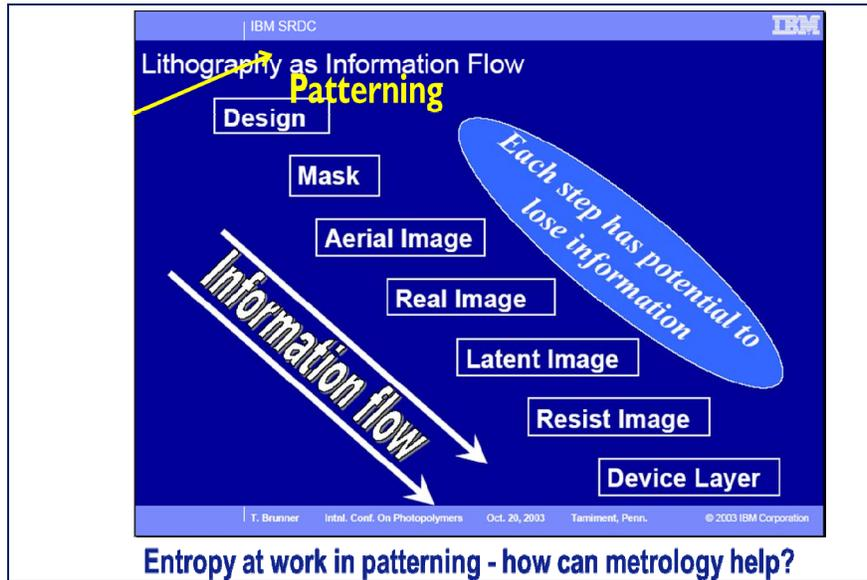
Figure 13: Information Flow from Design to Device [39].
