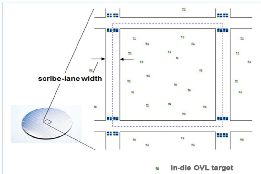
Figure 8: IC makers request additional intrafield overlay information.
