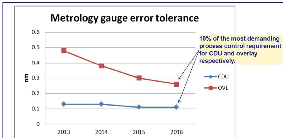
Figure 3: Metrology requirements in time of shrinking budgets.
