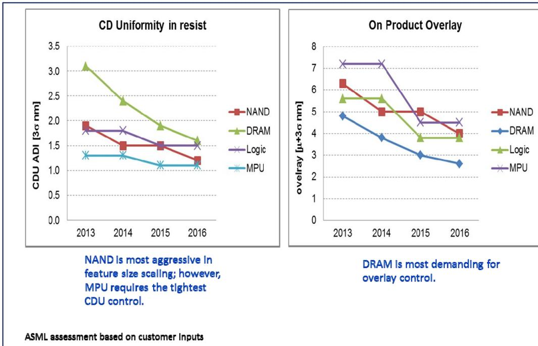
Figure 2: Estimated lithography process control requirements.
