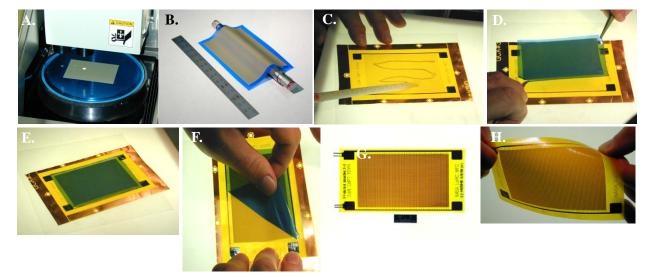
Figure 4. MFC fabrication; A. Slicing Wafer on dicing saw, B. Aligned rectangular fibers on Grip film, C. Applying adhesive to copper-etched Kapton<sup>®</sup> film, D. Placing fiber mat face down on adhesive, E. Bonded fiber-mat on etched Kapton<sup>®</sup> film, F. Peeling back Grip film, G. Finished MFC, H. Flexible MFC demonstration.
