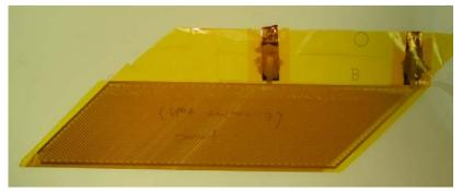
Figure 3. The Active Fiber Composite Actuator.
