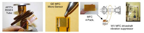
Figure 7. Examples of MFC prototype hardware, made by Smart Material Corp., and tested by external customers.
