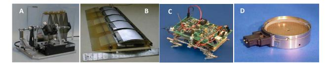
Figure 6. A THUNDER Piston-Motor (NASA), B. Dynamic Airfoil (NASA), C. Robot crawler (DARPA), D. Diesel Valve Injector (Caterpillar).
