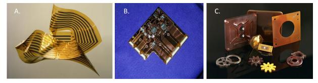
Figure 5. A. >0.5 mil Flex cable (NASA), B. Flexible high-speed multilayer adhesiveless A-D converter circuit (NASA), C. Mechanical parts (Imitec Inc.).
