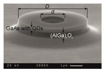
Figure 5. SEM image of QD microring laser ( $D = 6 \mu m$ ,  $d = 2 \mu m$ ).
