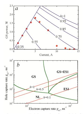
Figure 2. *L-I* curves for ground-state component (a): circles – experiment; lines – calculation for different ratio of hole-toelectron relaxation rates (*h*). Operation diagram of QD laser: heavy lines separates regions of different lasing regimes (NL – no lasing, GS – pure ground-state lasing, GS+ES1 – two-state lasing, ES1 – pure excited-state lasing); thin lines correspond to different *h* values.
