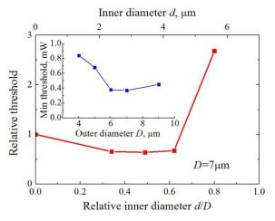
Figure 9. Room-temperature threshold (normalized to the threshold of the microdisk structure) as a function of inner diameter. Insert: the lowest threshold against the outer diameter.
