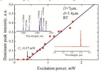
Figure 8. Intensity of the dominant mode against excitation power (symbols). Curve is a guide to the eye. Insert: luminescence spectrum below threshold (left) and above threshold (right).
