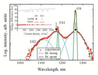
Figure 4. Emission spectrum: squares – experiment, solid curves – lasing emission, dotted curves – spontaneous emission. Insert: peak position vs current density: solid circles – GS lasing, open circles – ES1 lasing, solid curve – GS spontaneous emission, dotted curve – ES1 spontaneous emission.
