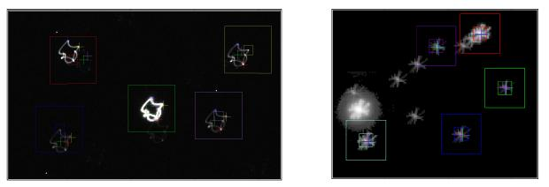
Figure 4 - Using MCC to accurately locate star centers when the gliph width is non-negligible
