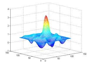
Figure 5 - MTI final result for a simulated magnitude 13 asteroid, after filtering
