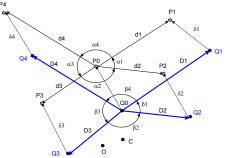
Figure 7 - Reference (distortion free) star pattern (Qi's) and the distorted and translated measured star pattern (Pi's).
