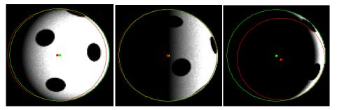
Figure 12 - Fitting circles to limb. Red: initial estimate, fitting an ellipse to an initial blob (phase compensation). Green: true circle.
