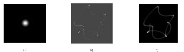
Figure 3 - a) PSF, b) glyph (or LOS trace) (exagerated), c) convolution between PSF and glyph
