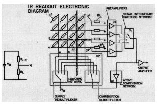
Figure 1. X-Y Electronic Addressing of IR FPAs [2, 15].
