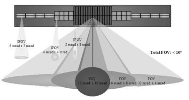
Figure 12. Block Scheme for improving single sub-pixel element resolution in large area signal extraction.
