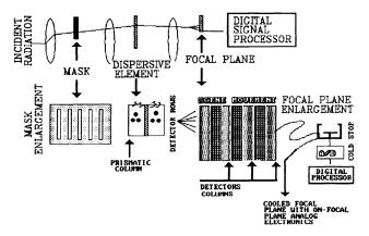
Figure 4. Multispectral reticule structured sensor.
