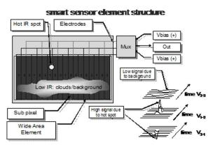
Figure 6. Detection of Point Source Target in presence of high clutter unwanted signals with increased resolution obtained by a 3 differential electrodes: This 3 electrodes structure was repeated 8 times within large area 1024 FPAs sensor elements.
