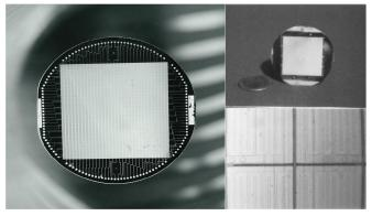
Figure 8. IR FPAs (1024 sensors, each one with 3x8 sub-pixels) Elettronica Spa Rome - Italy 1976.
