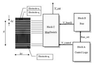
Figure 7. Block Scheme for improving single sub-pixel element resolution in large area signal extraction.
