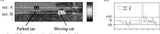
Figure 13. Thermal Imaging (a) and Smart Sensor Signal (b).
