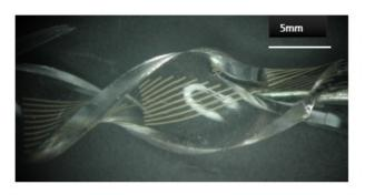
Figure 7. C-NCP electrodes fabricated via micromolding from PDMS filled with Ag nanoparticles<sup>38</sup>. Substrate has been twisted to show flexibility.
