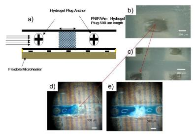
Figure 5. Mechanically-flexible plug-type PNIPAAm hydrogel valve with W-doped PDMS C-NCP, or flexible PCB metal, flexible heater element: a) schematic of valve showing subcomponents of device; b,c) hydrogel plug microfabrication via micromolding; d) normally-closed valve operation with heater off; e) open valve with heater on showing fluid flow from left to right (adapted from<sup>10</sup>).
