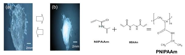
Figure 2. PNIPAAm hydrogel in: a) cooled, swollen state; b) heated, un-swollen state<sup>6</sup>.
