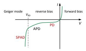
Figure 4. Reverse bias operation of photodiodes may be divided into three regions: PD, APD, and SPAD. The gain is 0 in the PD region, linearly proportional to V in the APD region, and "infinite" in the SPAD region.
