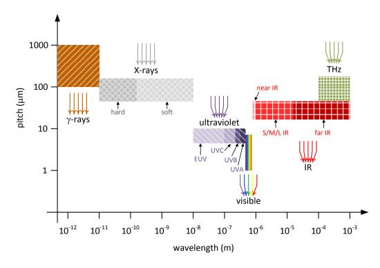
Figure 2. Variation of typical pixel pitch with imaging band. (All artwork is original.)
