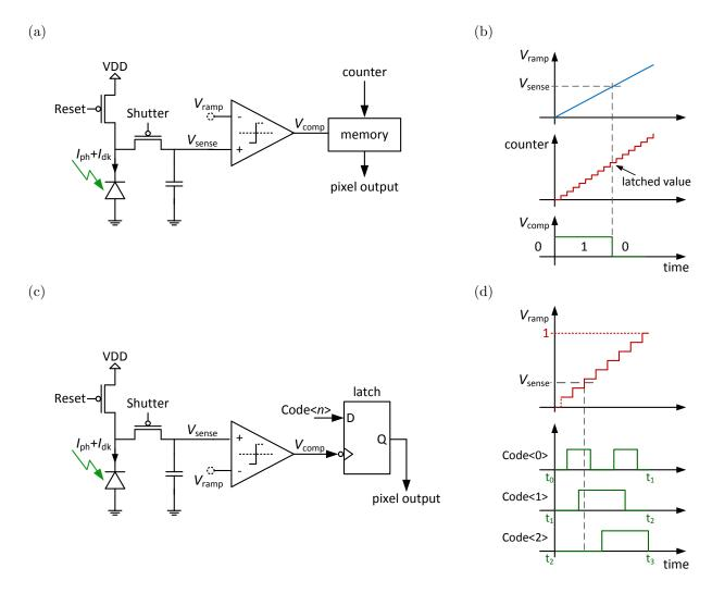
Figure 7. (a) In ramp-compare ADC pixels, erroneously called single-slope integrating ADC pixels, the detector output  $V_{\rm sense}$  is compared to an external ramp  $V_{\rm ramp}$ . (b) When  $V_{\rm sense} - V_{\rm ramp}$  changes sign, a ramp counter is latched in pixel memory. (c) In MCBS ADC pixels, there is only one bit stored per pixel, which saves area. (d) Ramp comparison is done multiple times in sequence, each time to resolve one bit of a code that identifies the ramp value.
