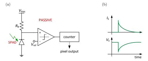
Figure 6. (a) A SPAD-based pixel with PQC has a serially-connected ballast resistor, a circuit that performs edge detection, and a counter. (b) Waveforms of the SPAD current and voltage, indicating Geiger operation, quenching, and reset.
