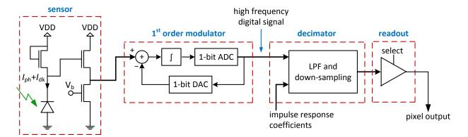
Figure 8. A true  $\Delta\Sigma$  ADC pixel, as shown, has both a modulator and decimator. The modulator oversamples and quantizes the ADC input, while shaping noise to high frequencies. The decimator filters the modulator signal and down-samples it to the Nyquist rate. In this schematic, a logarithmic sensor is shown, but linear sensors may also be used.
