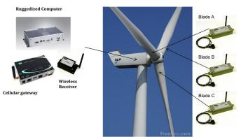
Figure 6. Components of a SHM system for turbine blade monitoring.
