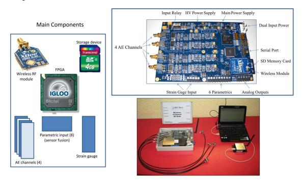
Figure 1. Components of the 1284 (4-channel wireless node), picture of the board (Rev 1.0) designed at Mistras, and the whole system connected to a laptop computer via a base station.
