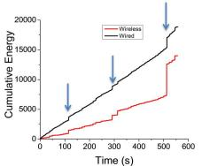
Figure 5. Cumulative AE energy as measured by the standard AE system (black) and the 1284 node (red) during the three point bending test. Notice the jumps (arrows) indicative of damage growth at different points during the test.
