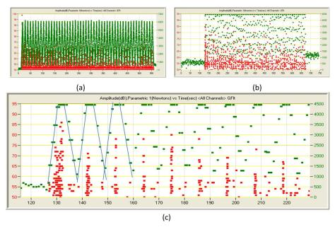
Figure 4. Data collected during the three point bending test, (a) Data collected with the standard AE system, (b) Data collected with the 1284 node, (c) Zoon of data collected with the 1284 node.
