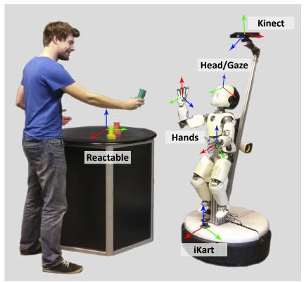
Figure 7. The EFAA human-robot interaction platform showing the multiple different reference frames that are integrated in the biomimetic control architecture (Reactable, iKart, Kinect, the two robot hands and its head).
