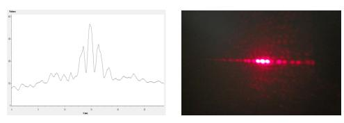
Fig. 5: Intensity pattern for 0.1mm width slits.
