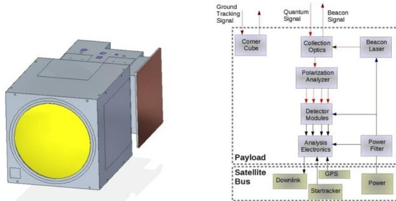
**Figure 3: Payload Solid Model (Left) and Block Diagram (Right).** Solid model shows outer casing (grey), collection lens (yellow) and radiator (brown).
