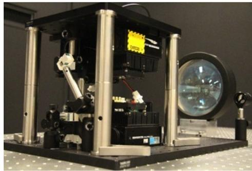
**Figure 4: Functional Test Setup Representative of NanoQEY Payload**
