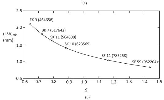
Figure 5. (a)The variation of CSF values for best lens shape with refractive indices, (b)The variation of (LSA)<sub>min</sub>'s with CSF values for best lens shape. The optical glasses having designations of 464658, 517642, 564608, 623569, 785258, and 952204 are indicated on both curves
