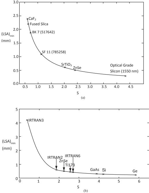
Figure 6. (a) and (b); the variations of minimum LSA's with CSF values of positive best lens shape for common IR lens materials which are used in IR regions. All lenses have the same paraxial focal length, central thickness, clear aperture, and operate at the same conditions of positive lenses in Fig.5.
