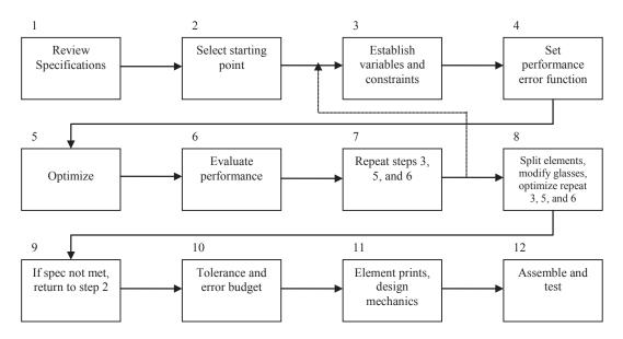
Figure 8. Lens design and optimization procedure.
