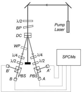
Figure 2. The experimental apparatus. Here  $\lambda/2$  denotes a half-wave plate,  $\lambda/4$  denotes a quarter-wave plate, BP denotes a birefringent plate, DC represents downconversion crystals, WP denotes an optional wave plate, and PBS denotes a polarizing beam splitter. A, A', B, and B' are lenses which focus light into optical fibers, which connect to the single photon counting modules (SPCMs).
