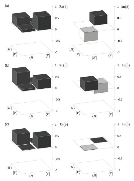
Figure 4. The real and imaginary parts of the density matrix for an entangled-state source. The measurements were conditioned on: (a) A being projected into state  $|L\rangle$ , (b) A' being projected into state  $|R\rangle$ , (c) either A or A'. Dark colored boxes correspond to positive values, while light colored boxes correspond to negative values.
