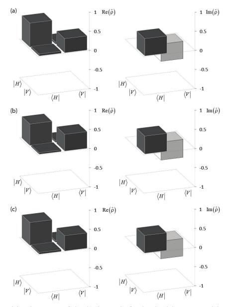
Figure 3. The real and imaginary parts of the density matrix for the signal beam prepared in state  $|L\rangle$ . The measurements were conditioned on idler detections at detector (a) A, (b) A', (c) A or A'. Darker colored boxes correspond to positive values, while lighter colored boxes correspond to negative values.
