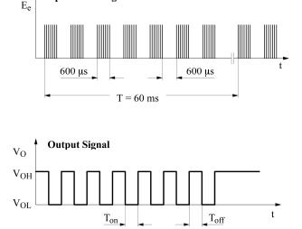
Figure 9: Optical signal and digital output signal [5]
