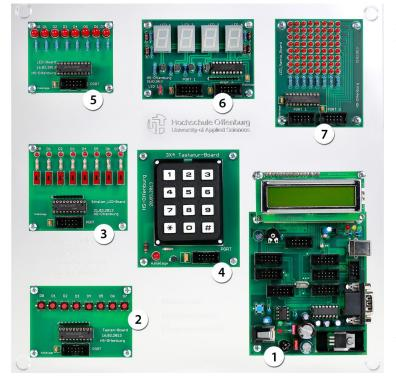
The development board is structured modularly. At the bottom right you find the microcontroller board with its LCD (1).
