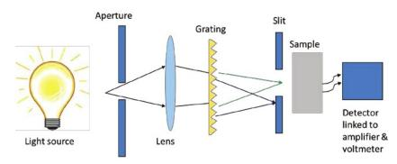
Figure 1. Basic components which can be employed in a simple spectrophotometer. \*patricia.forbes@up.ac.za; phone +27 (0)12 420 5426
