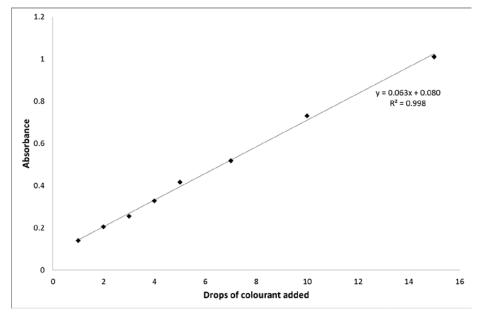
Figure 4. Calibration curve obtained with the SpecUP for blue food colourant dissolved in water.
