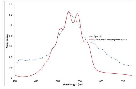
Figure 5. Comparison of the spectra of potassium permanganate obtained with the SpecUP and a commercial spectrophotometer.
