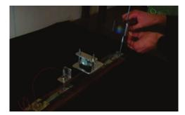
Figure 3. Changing the height of the sample cuvette in the SpecUP to vary the wavelength of light reaching the sample.
