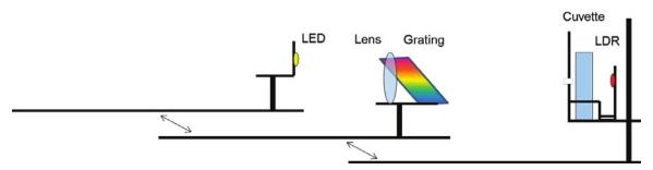
Figure 2. Side view showing the components of the SpecUP and their placement on retractable bars.
