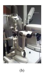
Fig. 1: (a) Image of the webcam with its adaptor; (b) Image of the slit-lamp with the webcam incorporated on the right hand objective.
