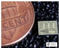
Figure 9: Four channel ASIC for driving DEA compared to the size a US penny.
