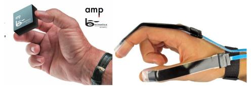
Figure 13: Motion capture controller (left) and soft sensor (right)
