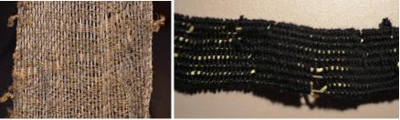
Figure 3: Nylon thermal actuators
