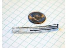
Figure 22: Carbon fiber infused EAP
