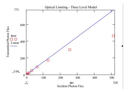
Figure 2. Optical limiting effect.
