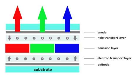
Figure 2. Schematic diagram of the OLED technology [16]-[19]
