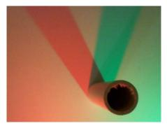
Figure 8. Colored shadows produced by using a red and a green LED that are spatially separated.
