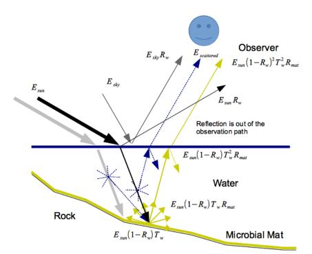
Figure 5. Sketch of the components included in a simple model of observed upwelling spectral irradiance  $E(\lambda)$ : diffuse skylight spectral irradiance  $E_{sky}(\lambda)$  reflected from the water (gray arrow); solar spectral irradiance  $E_{sun}(\lambda)$  reflected from the bottom (yellow arrow); and sunlight scattered within the water (dashed blue arrow). For clarity of the description, only a few paths of the upwelling light are shown.
