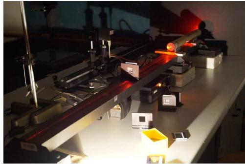
Figure 2. Set-up of the Fraunhofer optical experiment. The laser ray (He-Ne) crosses a small object, whose diffraction is projected on a faraway screen. The diffraction pattern corresponds to the Fourier transform.
